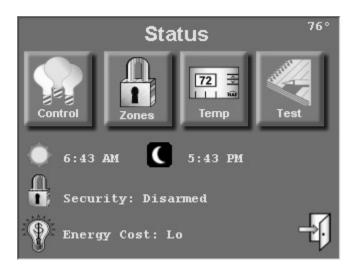
The main "Status" page displays the time of Sunrise and Sunset for the current day, current security mode, energy cost, and outdoor temperature (if applicable). According to your system configuration, not all icons may be visible (as shown above).
