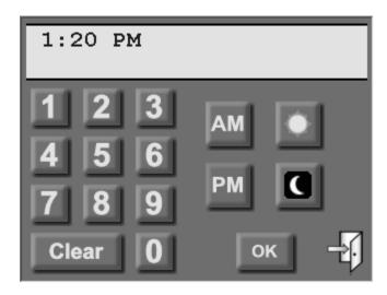
Enter the time (use either AM/PM or 24HR time format). Press the [sun] button for the "time of Sunrise" or the [moon] button for the "time of Sunset". Once complete, press the [OK] button to save time. If you make a mistake, press the [Clear] button and start over.
